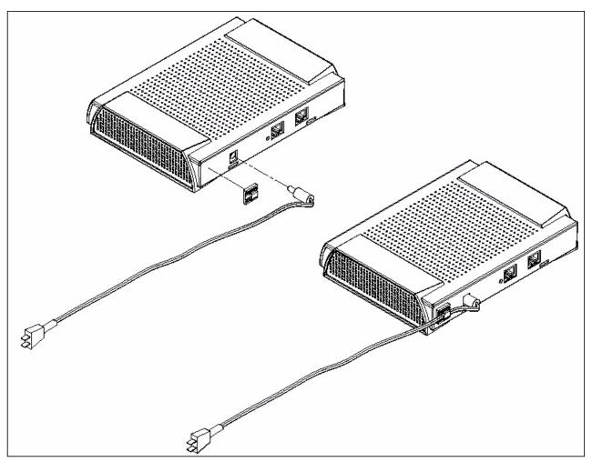
Figure 1 Power Kit Installation
